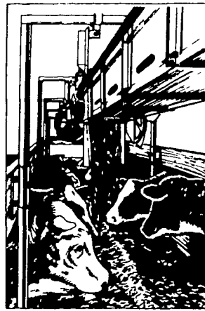
PATZ 166 OVERHEAD FEEDER exclusive self-aligning floating suspension
