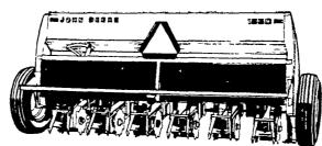
You know the value of interseeding pasture around here So come in to see the 1550 Powr-Till Seeder Design features start with a beefedup drivetrain featuring a T-drive gearbox, two slip clutches, high-capacity bearings and No 80 roller chain
