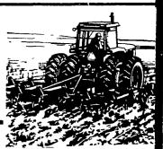
Twisted shovels rip moisture-absorbing grooves and blend in a soil-saving mulch to reduce runoff and resist wind
