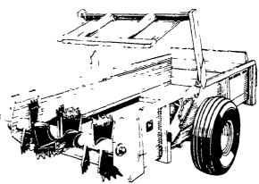
Spreading manure during winter is no fun, especially when the conveyor chain freezes down. And if it breaks, you have a real mess. John Deere now offers you a unique way to avoid spreader freeze-ups — the new 450 Hydra-Push Spreader with 217 cu. ft capacity (heaped, single beater) Hydraulic power — not a conveyor chain propels the material to the beater for spreading.
