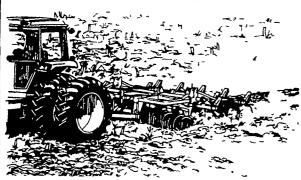
Combined tillage saves time, fuel and soil The curvature of 22-inch spherical blades works with the gang angle to cut heavy trash better than coulters Heavy-duty 11/2 x2-inch chisel standards shatter soil and mix residue, with power to spare And, adjustments are refined for fast, easy results
