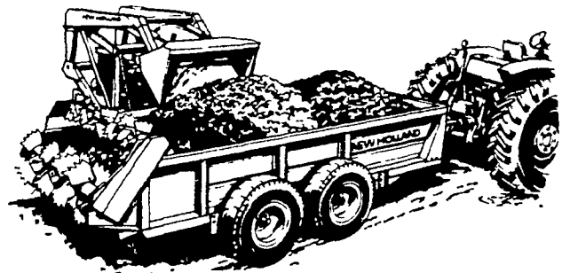
TANDEM AXLE BOX TYPE SINGLE OR DOUBLE BEATER TWO SIZES — 340 to 419 CU. FT.
