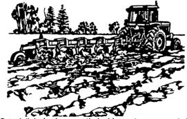
Get a full day's plowing with double-pivot spring-reset standards They'll slide over sloping obstructions or trip to clear ledge rocks then reset on the go But in extra hard ground, the standards remain firm to keep the bottoms in
