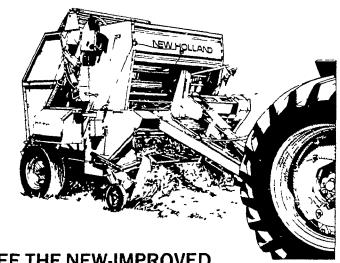
"847" ROUND BALER WITH ADJUSTABLE DUAL-COIL SPRINGS FOR HIGHER DENSITY BALES UNDER A VARIETY OF CROP CONDITIONS.
