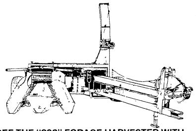
SEE THE "892" FORAGE HARVESTER WITH FLIP-UP FEED ROLL FOR EASY SHEAR BAR ADJUSTMENT. CUTAWAY MODEL WITH LIVE ELECTRONIC METAL DETECTOR WILL BE DISPLAYED.
