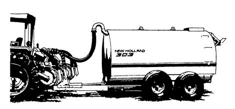
SEE THE "303" LIQUID TANK SPREADER WITH A CAPACITY OF 3,264 GALLONS. BROADCAST LIQUID MANURE IN SWATHS UP TO 40 FEET WIDE OR EQUIP IT WITH A TRACTOR MOUNTED INJECTOR.
