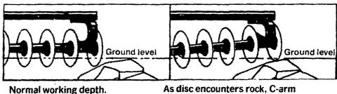
As disc encounters rock, C-arm compresses, allowing gang to ride up over obstacle.
