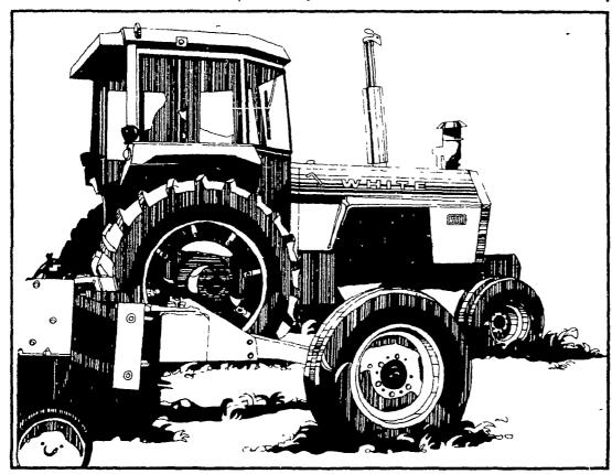
With 18 forward speeds in three shift-on-the-go power ranges, hydrostatic power steering plus optional power front axle, the 2-85 and 2-105 give you flexibility equal to the biggest 2-wheel drive tractors.
