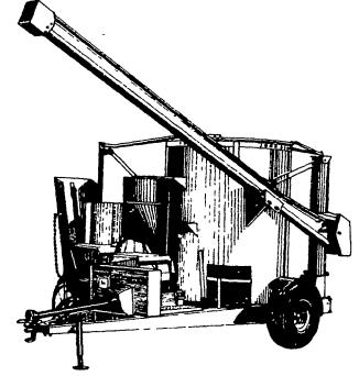
John Deere engineers designed the 700/750 Mixers to withstand tough grinding. These mixers come equipped with a 1000-rpm PTO, 20-inch-wide hammer mill, 64 hammers, and a 703-square-inch screen to allow feed to be ground fast. See us today for a 2or 3-ton mixer.
