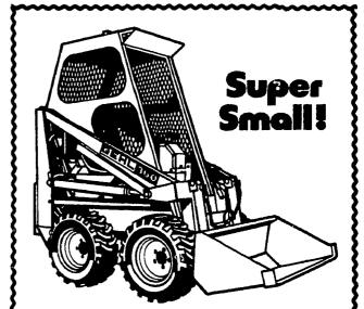
Gehi's new 360 loader – just under 36" wide! Gets in and out of the tightest spots And just two simple T-bars give you all the moves Hydrostatic drive 550# lift rating 16 hp Onan engine quick change attachments overhead guard all standard equipment
