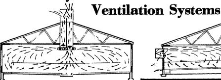
A unique air blending process provides even temperatures and controlled, draft-free air flow.
