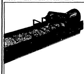
Double #55 Chains with 15" Oak Wood slats Carry Feeding Material in a 20" Wide Conveyor Standard Conveyor length is 16 ft. Shorter units are made to accommodate every requirement. Hopper (not shown) for input of feed material is available and will fit on top where needed Extra slack in conveyor chain can be adjusted at drive end Bottom Side Conveyor with Chain Return on top available Incline-to level Units made to order
