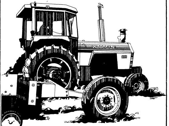
With 18 forward speeds in three shift-on-the-go power ranges, hydrostatic power steering plus optional power front axle, the 2-85 and 2-105 give you flexibility equal to the biggest 2-wheel drive tractors.
