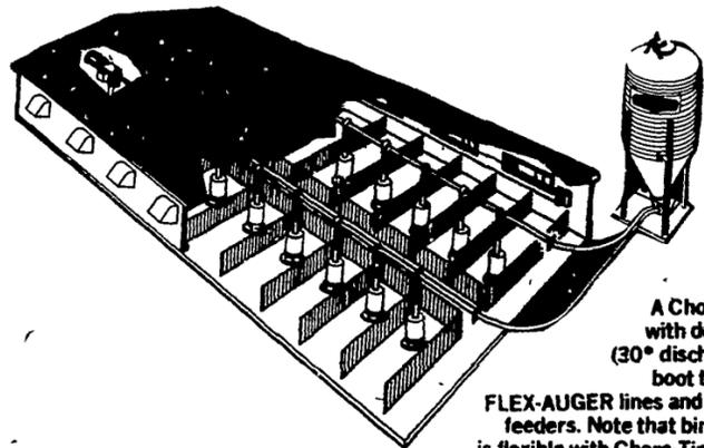
A Chore-Time bin with double outlet (30° discharge angle) boot to serve two FLEX-AUGER lines and two rows of feeders. Note that bin placement is flexible with Chore-Time systems.
