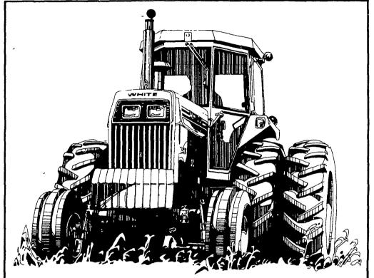
The exclusive 18-speed 3x6 Over/Under Transmission, inboard planetary final drives and closedcenter hydraulics are all standard performance features on the 2-135, 2-155 and 2-180 Field Boss Tractors.
