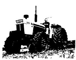
Case 1210 4-wheel drive. Boosts traction dramatically on heavy drawbar or loader work. Engage or disengage front wheel drive on the go in most condition. Especially adapted to rice farming, wild rice, wood work, tree farming etc. 65 HP. with canopy 1700 Hrs., reconditioned. Weights not incl. in price.
