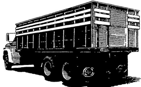
■ One-piece roll formed steel sides with built in tarp rail Available in 28", 40" and 52" extra-capacity heights all with maximum corrugation for maximum strength
