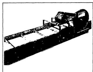
Double #55 Chains with 15" Oak Wood slats Carry Feeding Material in a 20' Wide Conveyor Standard Conveyor length is 16 ft. Shorter units are made to accommodate every requirement Hopper (not shown) for input of feed material is available and will fit on top where needed Extra slack in conveyor chain can be adjusted at drive end Bottom Side Conveyor with Chain Return on top available Incline-to-level
