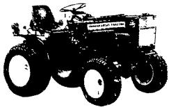
All NEW Shift On-The-Go. Live PTO. Powerful, troublefree 18 HP 3-cylinder Yanmar Diesel, 2 WD & 4 WD.
