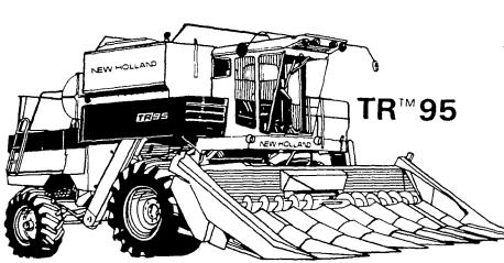
240 Bu. grain tank; 196 HP Caterpillar Diesel engine
