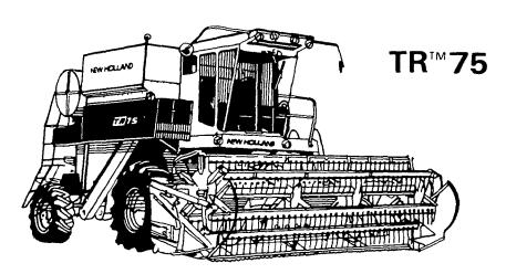
140 Bu. grain tank (190 Bu. with extensions):145 HP turbo charged Ford Diesel engine
