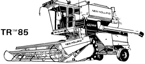
190 Bu. grain tank; 168 HP Caterpillar Diesel engine
