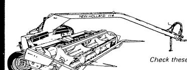
Pivot-tongue frame on the Model 114 lets you tow the windrower on either side of the tractor for cutting, or directly behind for transport. Cut both ways in the same field Choice of 12- or 14foot headers
