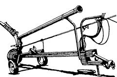
Pumps any size lagoon with 2·1 slope wall so you don't need docks or loading platforms. Delivers 5,500 gallons per minute. Driven at 540 RPM from tractor PTO Heavy-duty 25-inch impellor. 25' length, with optional extension to pump the deepest pits. Loading pipes and hydraulics included
