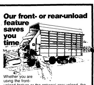
unload feature or the optional rear-unload, the John Deere 714A and 716A Forage Wagons save you forage harvesting time A fast 11 5-fpm conveyor speed lets you empty 593 cubic feet from the 714A and 677-cubic-foot payloads from the 716A in a hurry See them today
