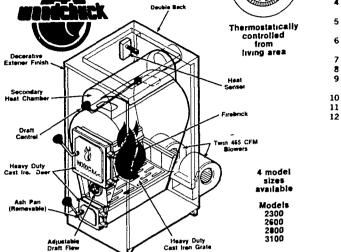
struction 2 High output 930 CFM blowers 25% more heat exchanger sur face area than most furnaces 4 Large cast iron fuel and ash doors w/ash tray 5 Long life circular heat exchang er design 6 All Honeywell controls sup plied Available Coal Shaker Grate All wiring hook ups supplied Living area thermostat opera tion available 10 Double back with 2 air space 11 All models successfully tested 12 Fully warranted
