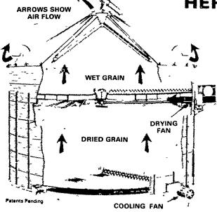
As wet grain enters the top of the bin, it flows into the upper drying chamber as harvested, with no need for a wet holding bin This upper chamber holds up to 4 feet of wet grain (2250 bushels)
