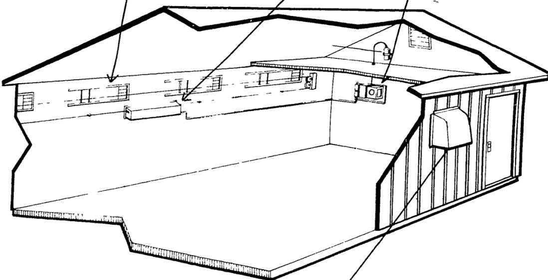
Four basic components go into the makeup of this ventilation system: the fan, the inlet, the air inlet power pack, and the controls. Coordinated, these four basic components can provide you with better conversion and performance by removing stresses due to lack of oxygen, excess humidity, noxious gases and temperature extremes.
