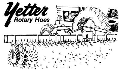
High speed cultivation saves energy! The Yetter Rotary Hoe releases caking, reactivates chemicals in dry soil, weeds and cultivates crops up to 8" high, all at 12 mph
