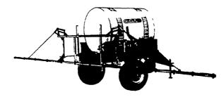
**CENTURY** Helps Provide Accurate Fertilizer Spraying One Unit In Stock Equipped With The Following: 10 Row Heavy Duty Boom With Shock Absorbers. 500 Gal. Tank on Heavy Duty Trailer with 11Lx15 Flotation Tires, with Agitator and PTO Centrifugal Pump and 3 way Valve with catwalk and guard
