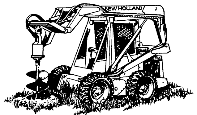
DIG POST HOLES
