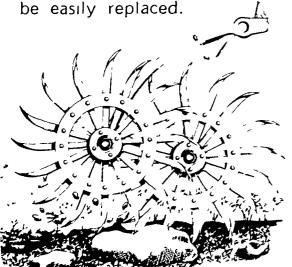
Each wheel is mounted on its own arm, free to follow the ground contour for maximum weed control and crust busting
