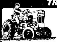
Breeze thru your Work! Power King's all gear drive delivers nearly 100% of horsepower to the wheels Available with 12 14 and 18 hp engine, and up to 19' cultivating clearance Handles 4 and 5 mowers 2" plow, 32" tiller 42" and 48 'snowblowers, 4 dozer,
