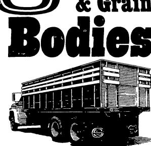
One-piece roll formed steel sides with built in tarp rail Available in 28", 40" and 52" extracapacity heights all with maximum corrugation for maximum strength
