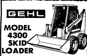
Hydrostatic Drive, Self-Leveling Loader, 30 H.P., 700x15 Tires, 65 inch Material Bucket
