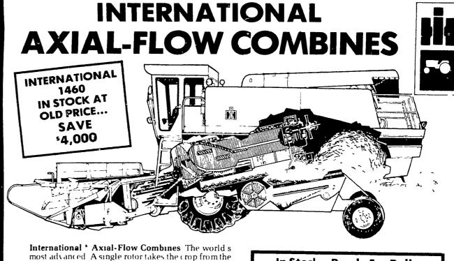
feeder and whirls it in a spiral path through the machine. The crop makes multiple cotacts between rotor rasp bars and rotor cage concaves for thorough threshing. It is simplicity itself. There is no cylinder. no cylinder beater or beater grate, no straw walker and no rack. You harvest more grain with less kernel damage. More than that. Axial Flow combines give you greater productivity reliability and easier serv iceability
