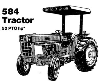
The 584 tractor combines big, responsive power and quick, landling to make every job go faster and eas pull for plowing and disking independent 540 PTO for baling and forage harvesting . plus all the hydraulic power you need for loading Utility and row-crop models
