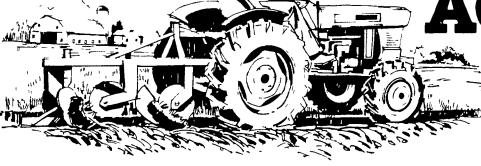
17-HP L185DT with four-wheel drive, and moldboard plow.
