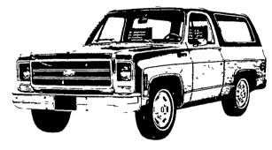
250 6 Cylinder, 4 Speed Synchromesh Trans., Free Running Hubs, Power Steering, Power Brakes, Folding Seat, Fiberglass Cab...
