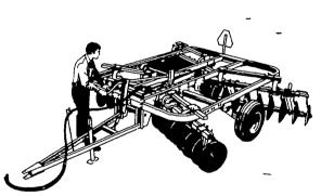
You can leave the wrenches in the tractor when you level this new 115 Level-ActionTM Disk. Finetune fore/aft leveling by turning the hand crank above the hitch. In many fields, this simple adjustment is the only one you'll need to make.
