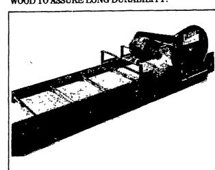
Double #55 Chains with 15" Oak Wood slats Carry Feeding Material in a 20" Wide Conveyor Standard Conveyor length is 16 ft Shorter units are made to accommodate every requirement Hopper (not shown) for input of feed material is available and will fit on top where needed. Extra slack in conveyor chain can be adjusted at drive end Bottom Side Conveyor with Chain Return on top available Incline-to-level Units made to order
