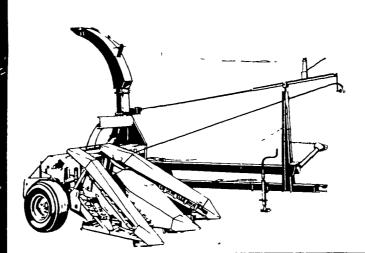
The Sperry New Holland Model 770 forage harvester features a 12-knife cutterhead and PTO-driven power knife sharpener You also get
