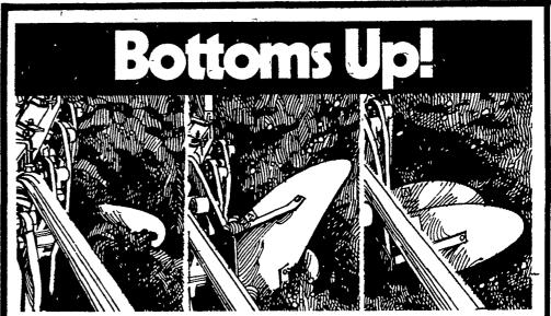
Come see Monoframe plows with Bump and Run hydraulic reset bottoms which lift over buried objects and reset automatically Look into the Allis-Chalmers 7bottom semi-mounted plow. It gives you 18-inch furrows in a 12-foot wide cut Plugging is all but eliminated thanks to a full
