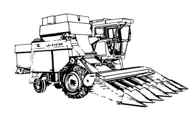
The new model 818 is bigger, more rugged and has a larger harvesting capacity. In fact 33% more capacity than the current 717 Combine. This new generation Combine has a 165-bushel grain bin, plus a wide 48-inch cylinder. It is designed to be used with the 801 Power Unit, FAS-TACH corn heads, and bean/grain platforms, with changeover from corn harvesting to bean harvesting in just minutes. The 818 Combine... built in the finest New Idea tradition.
