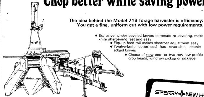
• Exclusive under-beveled knives eliminate re-beveling, make knife sharpening fast and easy Flip-up feed roll makes shearpar adjustment easy
