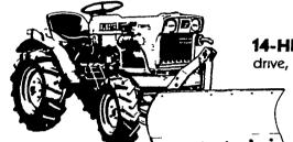
14-HP B6100 DT with four-wheel drive, and front blade
