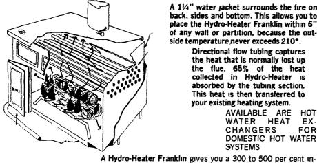
A 1¼" water jacket surrounds the fire on back, sides and bottom. This allows you to place the Hydro-Heater Franklin within 6" of any wall or partition, because the outside temperature never exceeds 210\*.
