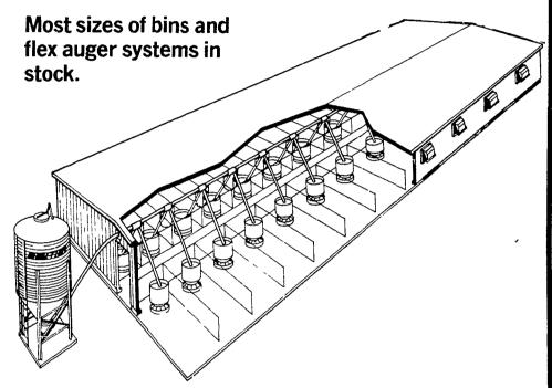
Both rugged and versatile, the Flex-Auger System easily adapts to most hog feeding operations. The Chore-Time centerless auger delivers feed from bulk bin to all feeders located throughout the house. Much of the labor required with other methods is eliminated. The Y outlet drop assembly (illustrated above) or single units can be installed in most any position desired. Feed level is easily controlled by adjusting the height of the drop.
