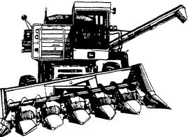
On-the-go, automatic separator leveling from feeder house through cleaning shoe is yours with a -SideHill 6600 Combine. As the separator levels on slopes to 18 percent, the header pivots to parallel the ground. Keeping the separator level maximizes your crop savings because no material drifts to the downhill side as with a conventional combine. And to master hilly fields, you get a 128 hp 404 cubic inch diesel engine. The cylinder is 44 inches wide.
