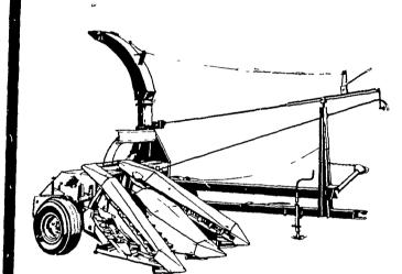
The Sperry New Holland Model 770 forage harvester features a 12-knife cutterhead and PTO-driven power knife sharpener You also get
