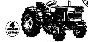
Model L245DT Here's more traction and versatility from the new Kubota line Rugged, yet agile four-wheel drive model with outstanding the agile of the content of the conten and great lugging power Powered by a water-cooled 25HP, 3-cylinder diesel engine. Implements are handled with ease by the powerful hydraulic lift system Plus PTO's, standard
