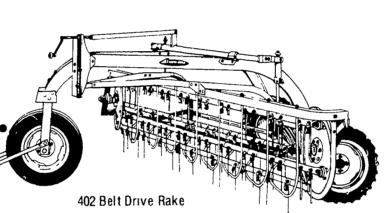
Smoothly, quietly, it rakes an exceptionally clean 8-1/2 foot width with minimum leaf shattering and builds fluffy, uniform windrows. The straight axle design, working with the spring suspension with friction brake, reduces basket bounce, even on rough terrain.
