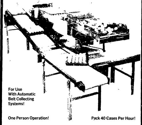
The spring cushion conveyors, for more gentle and positive egg handling, take the eggs thru the disc type orientors, which softly place them, points facing the same direction, into our blue cups. Here the operator merely places the package over the eggs.
